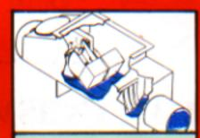
When water level in street sewer recedes to normal, flood gate opens automatically and building drainage returns to normal.
