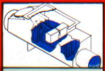
Rising water in sewer line lifts the float. This in turn operates the flood gate, completely sealing off the main sewer line, preventing backflow.
